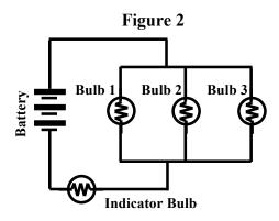
Then the students unscrew both Bulb 1 and Bulb 2 from their sockets. They observe that Bulb 3 remains lit. They also observe that the Indicator Bulb is dimmer than it was with two and with three branched bulbs.
