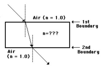
4. Cal Culator is performing experiments to determine the index of refraction of two unknown materials. Cal determines that the light follows the paths as shown on the diagrams below. Use this path, a protractor, a calculator and Snell's Law to determine the index of refraction of the unknown material. Show all your work in the space beside the diagram.
