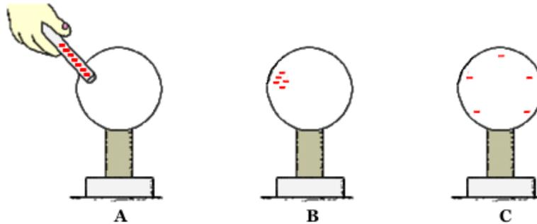
A: A teacher holds a negatively charged metal bar by its insulating handle and touches it to a metal sphere (attached to an insulating stand).
