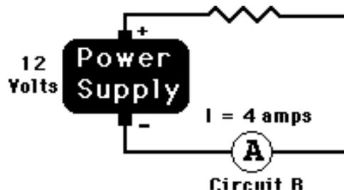
10. Use arrows to show the direction of conventional current flow through the following circuits and use the  $I = \Delta V / R$  equation to fill in the blanks.
