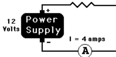
10. Use arrows to show the direction of conventional current flow through the following circuits and use the  $I = \Delta V / R$  equation to fill in the blanks.
