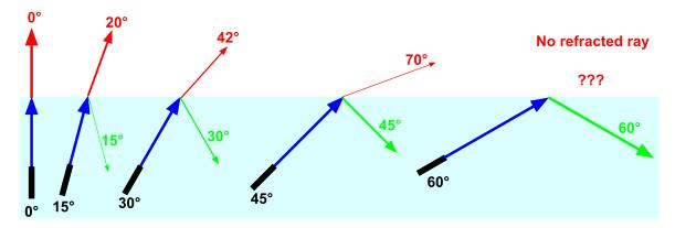
As the angle of incidence is increased from 0° to larger angles, the angle of refraction approaches 90° until finally a refracted ray is no longer seen. The light undergoes reflection ONLY.
