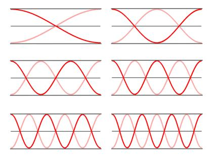
The fundamental or first harmonic frequency of an open-end air column is 60 Hz. The same air column is capable of vibrating with several other standing wave patterns. Identify the standing wave pattern for the harmonic that has a frequency of 180 Hz.
