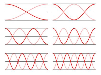
The fundamental or first harmonic frequency of an open-end air column is 120 Hz. The same air column is capable of vibrating with several other standing wave patterns. Identify the standing wave pattern for the harmonic that has a frequency of 240 Hz.
