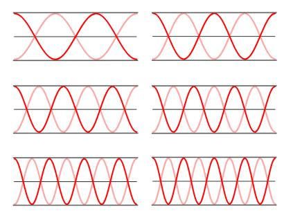
The fundamental or first harmonic frequency of an open-end air column is 60 Hz. The same air column is capable of vibrating with several other standing wave patterns. Identify the standing wave pattern for the harmonic that has a frequency of 420 Hz.
