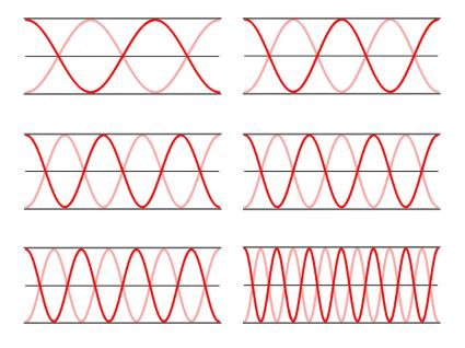
The fundamental or first harmonic frequency of an open-end air column is 120 Hz. The same air column is capable of vibrating with several other standing wave patterns. Identify the standing wave pattern for the harmonic that has a frequency of 720 Hz.
