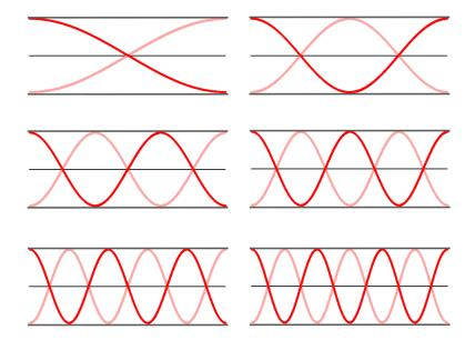
An open-end air column has a length of 60 cm. Identify the standing wave pattern for the harmonic that has a wavelength of 30 cm.
