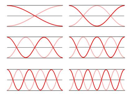
An open-end air column has a length of 80 cm. Identify the standing wave pattern for the harmonic that has a wavelength of 32 cm.
