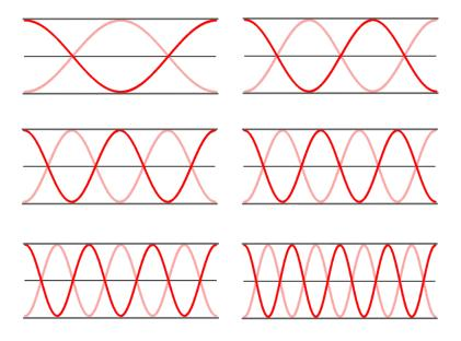
The fundamental or first harmonic frequency of an open-end air column is 120 Hz. The same air column is capable of vibrating with several other standing wave patterns. Identify the standing wave pattern for the harmonic that has a frequency of 480 Hz.
