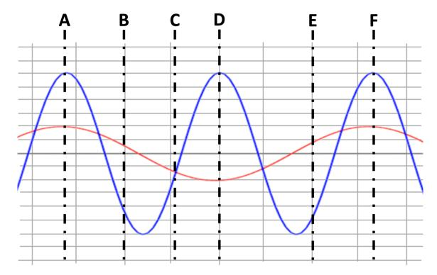
Constructive Interferene Points: A, C, and F
