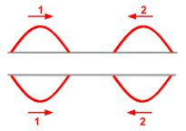
**Destructive Interference:** occurs when the displacement is in opposite directions.
