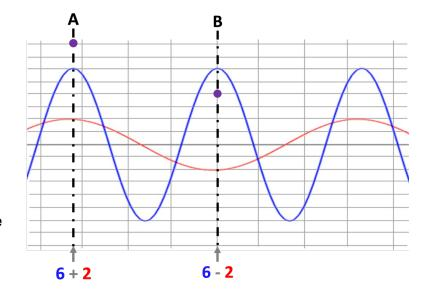
By applying the principle of superposition to several points along the medium, you can determine the displacement at each location and an estimated shape of the resultant wave at that moment in time. This is shown in the diagram.
