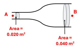
How does the volumetric flow rate ( $\bf Q$  in m³/s) and the flow velocity ( $\bf v$  in m/s) at  $\bf B$  compare to that at  $\bf A$ ?
