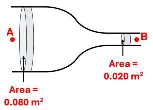
How does the volumetric flow rate ( $\mathbf{Q}$  in m<sup>3</sup>/s) and the flow velocity ( $\mathbf{v}$  in m/s) at  $\mathbf{B}$  compare to that at  $\mathbf{A}$ ?
