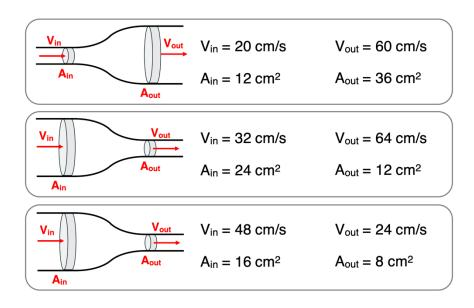
Fluid in a pipe flows between two sections with different cross-sectional areas. The areas (A) and flow velocities (V) are listed. Identify all situations that violate the law of conservation of mass.
