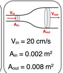
Consider the three situations in which fluid in a pipe flows between regions with a different cross-sectional area (A). Rank the V<sub>out</sub> values for the three situations.
