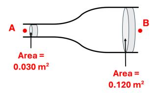
How does the volumetric flow rate ( $\mathbf{Q}$  in m<sup>3</sup>/s) and the flow velocity ( $\mathbf{v}$  in m/s) at  $\mathbf{B}$  compare to that at  $\mathbf{A}$ ?
