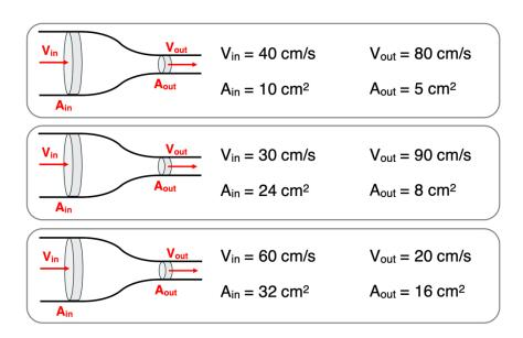
Fluid in a pipe flows from a wide to a narrow section. The cross-sectional areas (A) and flow velocities (V) are listed. Identify all situations that violate the law of conservation of mass.
