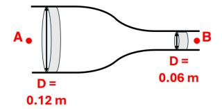
How does the volumetric flow rate ( $\mathbf{Q}$  in m<sup>3</sup>/s) and the flow velocity ( $\mathbf{v}$  in m/s) at  $\mathbf{B}$  compare to that at  $\mathbf{A}$ ?
