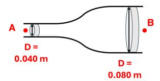
How does the volumetric flow rate ( $\mathbf{Q}$  in m<sup>3</sup>/s) and the flow velocity ( $\mathbf{v}$  in m/s) at  $\mathbf{B}$  compare to that at  $\mathbf{A}$ ?
