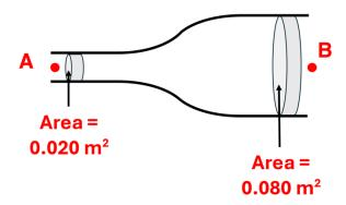
How does the volumetric flow rate ( $\bf Q$  in m³/s) and the flow velocity ( $\bf v$  in m/s) at  $\bf B$  compare to that at  $\bf A$ ?
