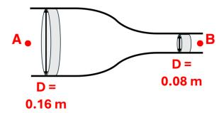
How does the volumetric flow rate ( $\bf Q$  in m³/s) and the flow velocity ( $\bf v$  in m/s) at  $\bf B$  compare to that at  $\bf A$ ?
