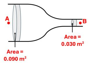
How does the volumetric flow rate ( $\bf Q$  in m³/s) and the flow velocity ( $\bf v$  in m/s) at  $\bf B$  compare to that at  $\bf A$ ?
