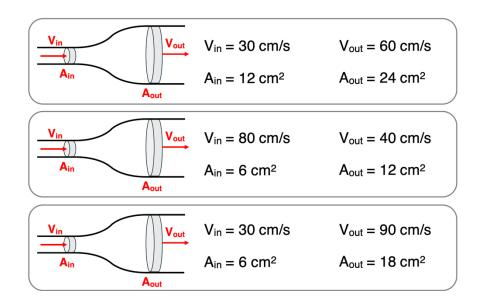
Fluid in a pipe flows from a narrow to a wide section. The cross-sectional areas (A) and flow velocities (V) are listed. Identify all situations that violate the law of conservation of mass.
