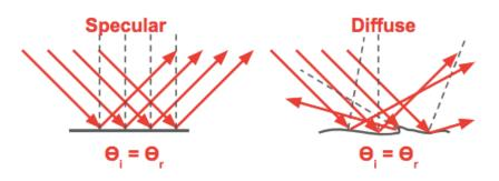
beam is not parallel to each other. Because of surface irregularities, not every ray encounters the same surface orientation.
